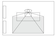
Lighting solutions for vertical visual tasks free of reflected glare: (from left to right): if the reflective surface is arranged transversely, the luminaires can be mounted in front of the excluded ceiling zone. If the reflective surface is arranged vertically, then next to
